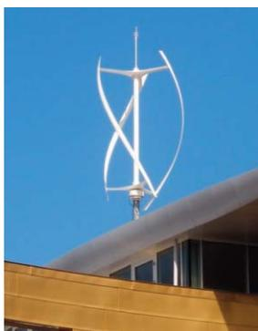
Average wind speed is a key factor to consider for any wind turbine installation and the recommended annual average wind speed for a location is 5 metres per second (11 mph). There are a number of factors that can affect wind speed such as nearby buildings, trees and the height of the turbine from the ground. An ideal location will have no significant obstructions such as tall buildings that are likely to either reduce wind speed or create a turbulent airflow.
